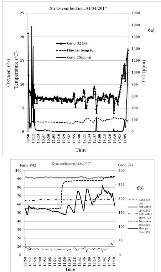
**Figure 6** - Time evolution of straw combustion in 4 April trial. Figure 6a) depicts the time variation of 3 variables in flue gas (concentrations of O<sub>2</sub>, CO and temperature). Figure 6b) depicts the time variation of oxygen concentration, cold and heated water temperatures and the temperature of the water in the top of storage tank
