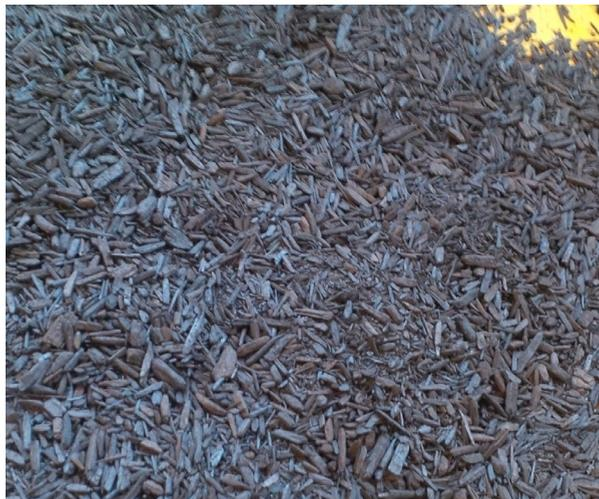
**Figure 1** - Torrefied pine tree wood chips produced at YGE – Yser Green Energy SA (Portugal)
