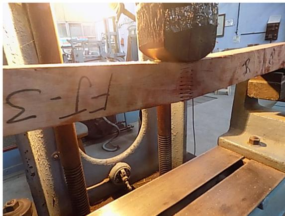
**Figure 1** - Photo of a finger-jointed *Eucalyptus* section under bending test
