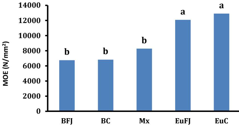
**Figure 3** - The Mean MOE of the different sets of samples studied
