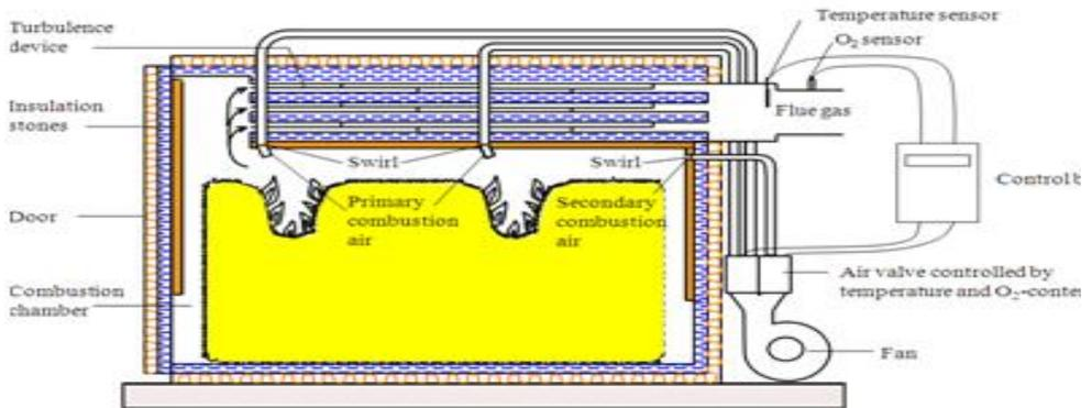
**Figure 3** - Diagrammatic representation of the straw boiler and burning
