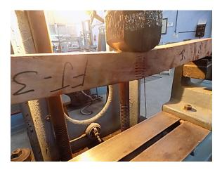
Figure 1 - Photo of a finger-jointed Eucalyptus section under bending test The results of static bending parameters obtained on the five sets of samples are given in Table 1
