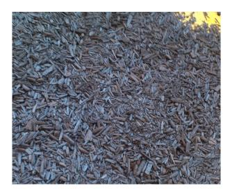
Figure 1 - Torrefied pine tree wood chips produced at YGE - Yser Green Energy SA (Portugal)
